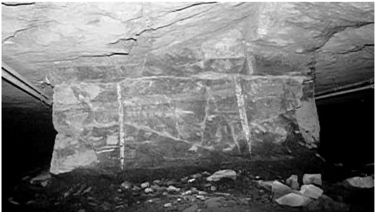
Figure 4.10 – Example showing pegmatite veining in a pillar. These are planar features, although often dislocated across the various chromitite seams
