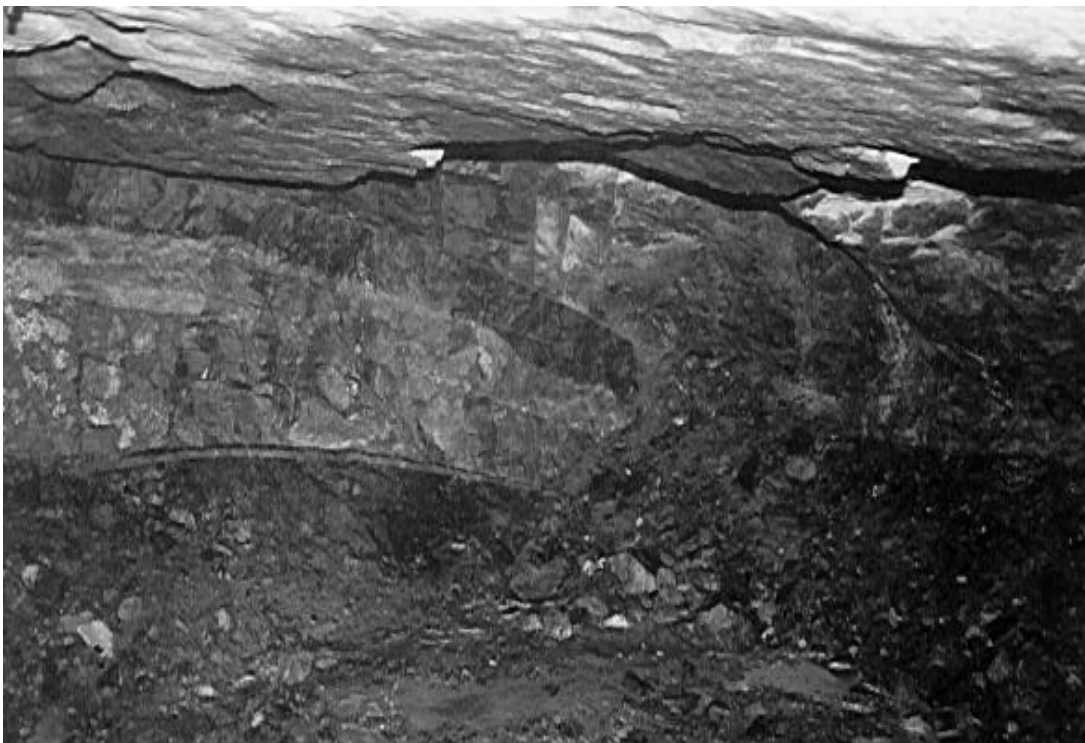
Figure 3.12 - Typical pothole showing rolling of the UG2 reef horizon in a platinum mine. Potholes are generally near circular or oval in plan and vary considerably in size from a few metres to hundreds of metres, with varying degrees of severity of roll. Mining has entered the hangingwall along the roll.
