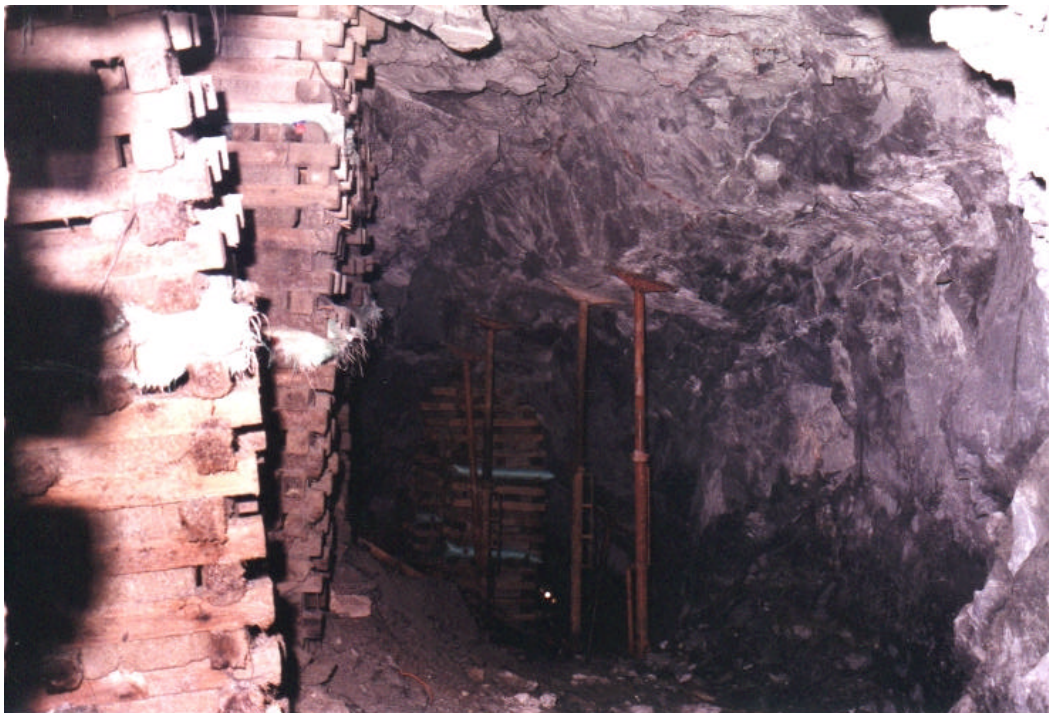
Figure 3.3: Loss of control in a VCR panel after encountering a roll. Reef is approximately 1 m thick at base of face (on the right), and 3 m of lava have fallen out. Tall packs and mechanical props are ineffective as support. The upper sketches explain the cause of the problems that arise with rolls. The high resulting stope face becomes prone to face-bursting in the hard, strong VCR lava.
