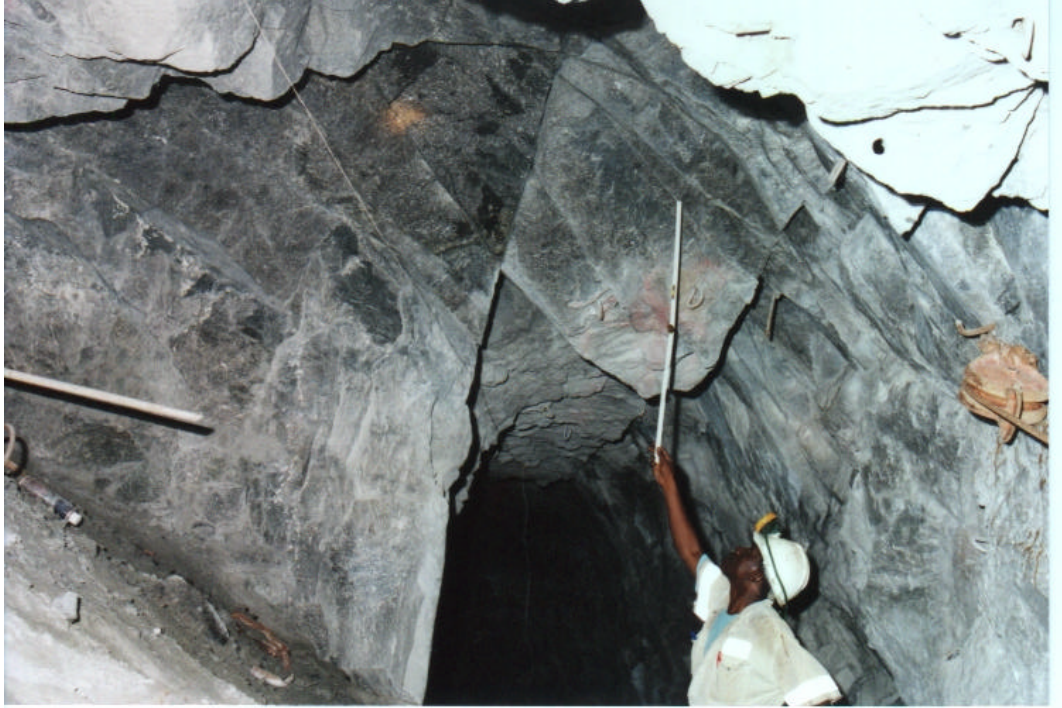
Figure 3.7 - Interaction of joints and a minor fault at shallow depth on the Merensky reef produce typical unstable wedges of ground in the otherwise massive rock mass. Example is at the face of a stope mining along a pre-developed reef drive.
