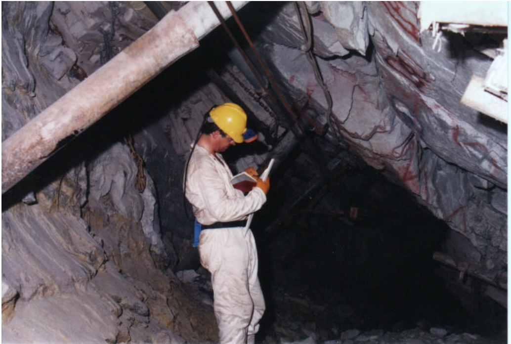
Figure 3.6 - Brows along a gully on Basal reef where bedding-bound blocks have collapsed. Rockprops are being used to control further collapse on the up dip side of the gully.
