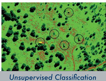
siderable difficulties dealing with the rich information content of high-resolution data (e.g. QuickBird). This produces inconsistent classification results and the software has difficulty in extracting the objects of interest. The success rate of detecting camouflaged objects, using this method, was 40%.
