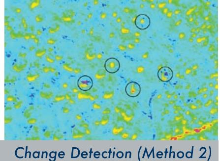
appears to perform generally better than other methods of change detection [1]. A major drawback is that seasonal changes reduce the probability of detection. During this exercise an EROS image was used as a reference image, and subtracted from the Quickbird image. The success rate of detecting camouflaged objects, using ID, was 56%.
