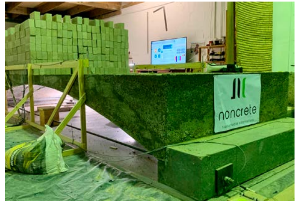
Doing more with less: The asymmetrical load testing of 12.8 kPa on a un-reinforced 5-meter span "nonCrete" funicular floor after 16 hours of uninterrupted loading - thereby exceeding European Building Code requirements. Undertaken in partnership with the Block Research Group, ETH Zurich – 2022
