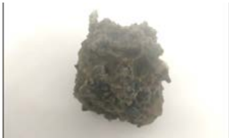
Figure 4-2: PC-dolomite specimen taken from the static HCl test after 350 hours
