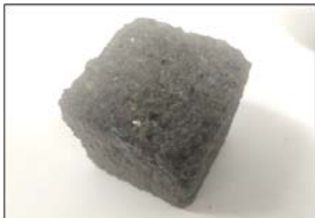
Figure 4-1: CAC-dolomite specimen taken from the static HCl test after 350 hours
