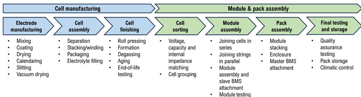
Figure 3: Lithium-ion battery manufacturing process steps from cells to pack assembly. Adapted from [17, 19].
