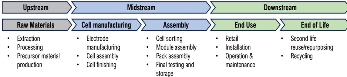
Figure 1: Lithium-ion battery value chain and associated activities. Adapted from [6].
