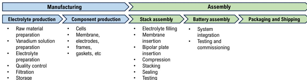
**Figure 5: Vanadium flow battery manufacturing process steps**
