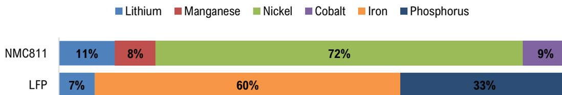
Figure 2: Metal composition of NMC811 and LFP cathode active materials. Adapted from [8].
