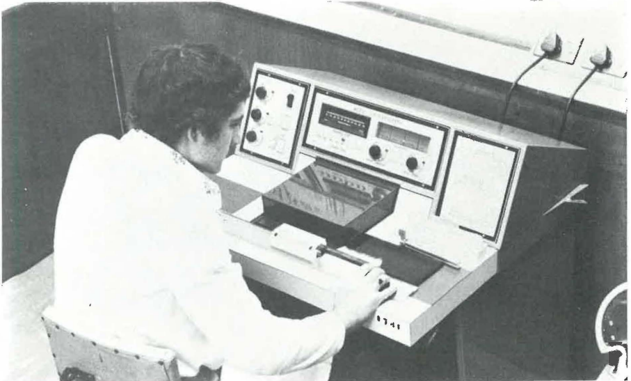
A Fibrograph, Model 330 in the cotton processing division's testing laboratory at SAWTRI
