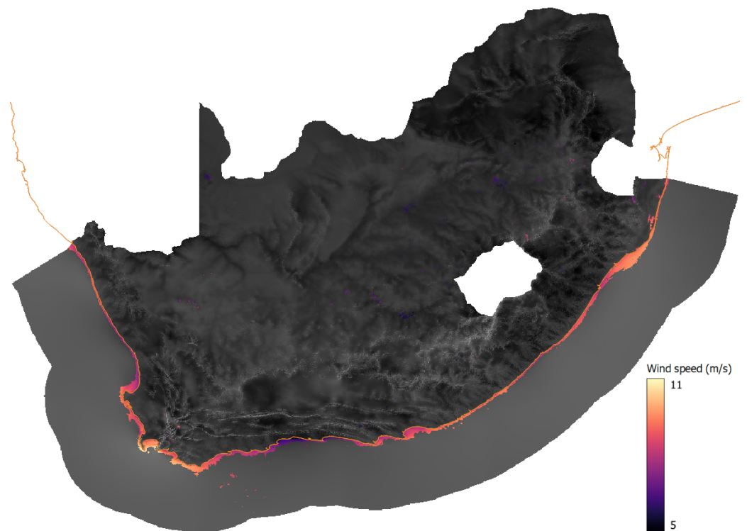
Figure 22. Average wind speeds at a 150 m elevation for ocean depths of 0 to −60 m.
