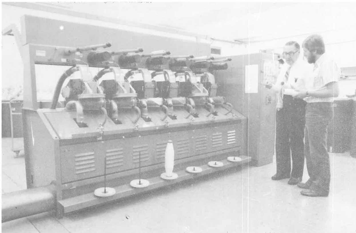
SAWTRI'S recently installed six-head DREF II OE spinning frame. Mr J. D. Spencer, Group Leader for Cotton Processing (left) discussing a technical point with a DREF installation technician from Dr Ernst Fehrer AG, Austria.
