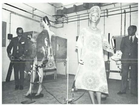
Among the interesting demonstrations of SAWTRI's cotton research, on May 1st, was one illustrating the Institute's successful application of flame retardancy treatment to cotton fabric. In the photograph it can be seen how untreated cotton is being consumed by fire while the treated fabric hardly burns at all
