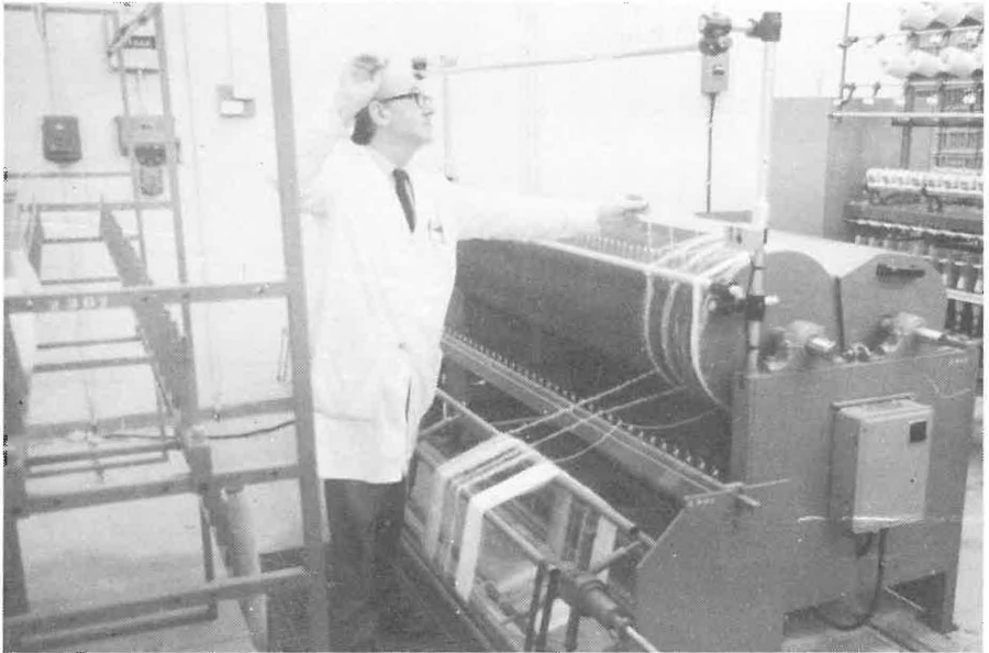
SAWTRI's Spinning Department recently had this Guma/GAR yarn brushing machine installed. This machine gives a raised or brushed effect on spun yarns
