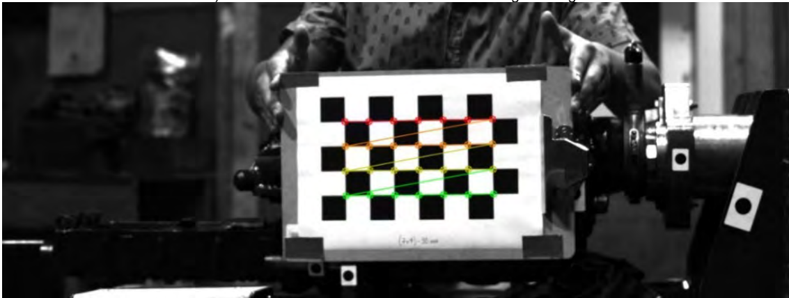
Fig. 2. Camera Calibration Checkerboard Corner Detection.
