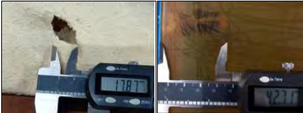
Fig. 11 Rubber projectile penetration through 1.1 mm Chamois (LHS) and into Gelatin Block
