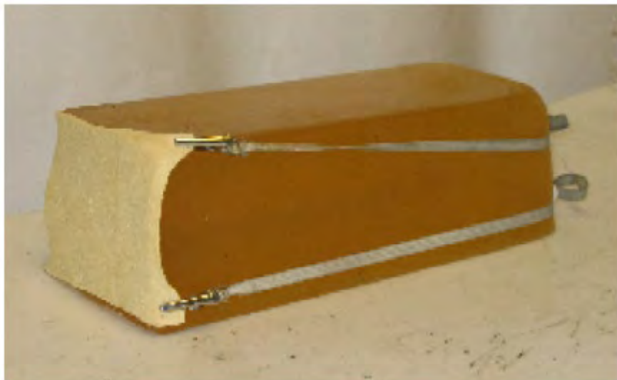
Fig. 6. Test setup for evaluation of skin and tissue surrogate materials [5]
