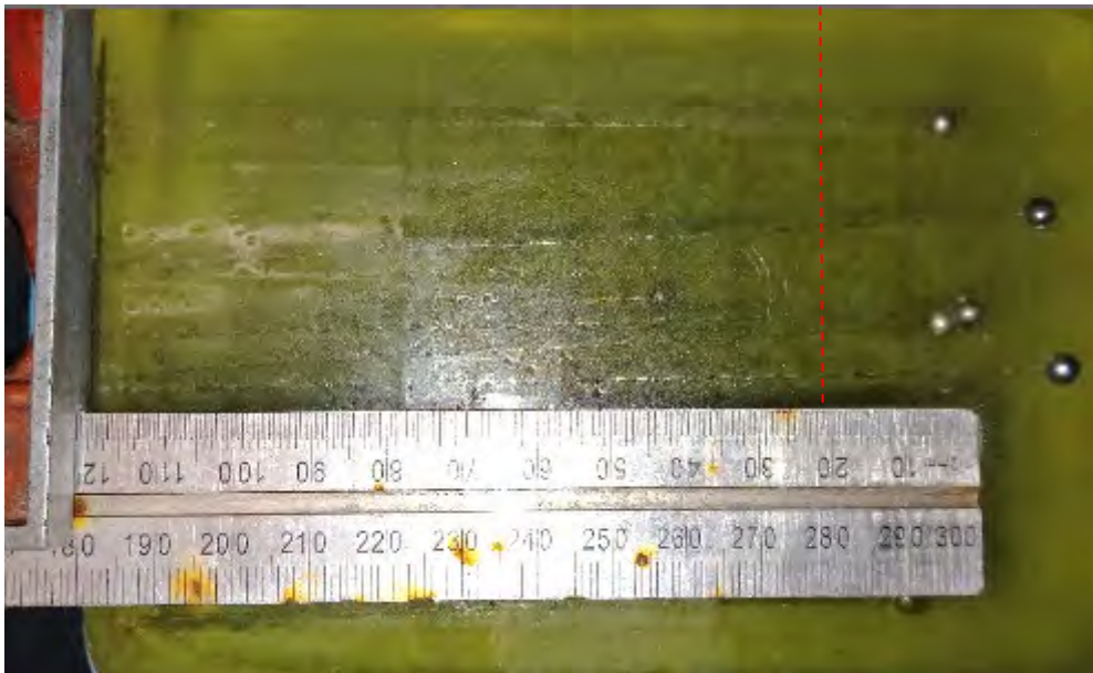
Fig. 8: BB Pellet depth of 112 mm at a velocity of 598 fps
