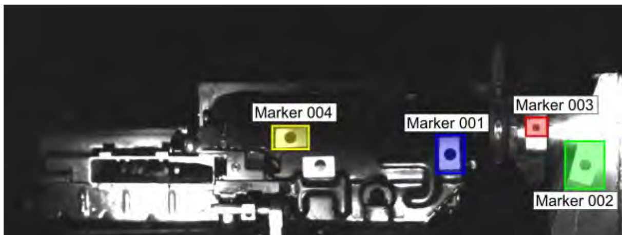
Fig. 4. Markers placed on the weapon and weapon mount.
