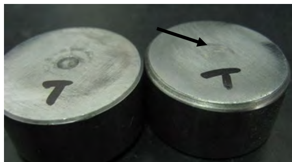
Fig. 5. Indentation Failure on the Temperature Cycle (right hand side).
