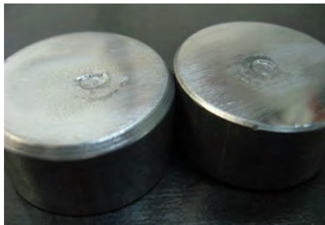
Fig. 4. Typical indentation of a Booster Relay on a witness block.
