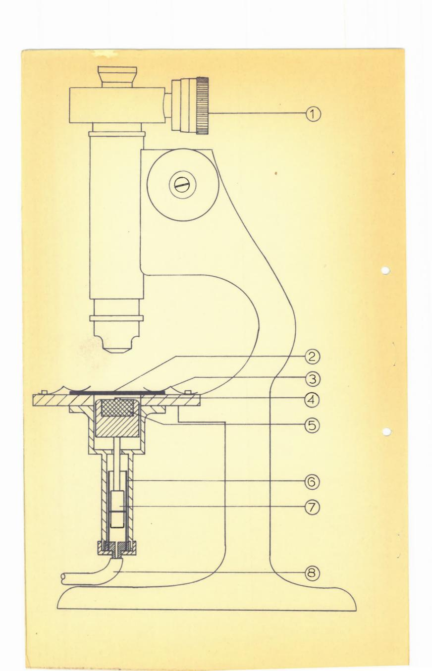
The condenser of the microscope was removed to allow accommodation for a small precision bore cylinder, (6) in <u>Figure 1</u>, and piston (7), which was fixed rigidly to the stage.
