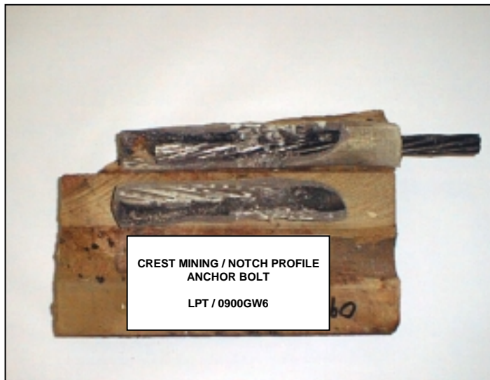
UNBULBED NOTCHED STRAND IN FASLOC RESIN (TEST 6)
