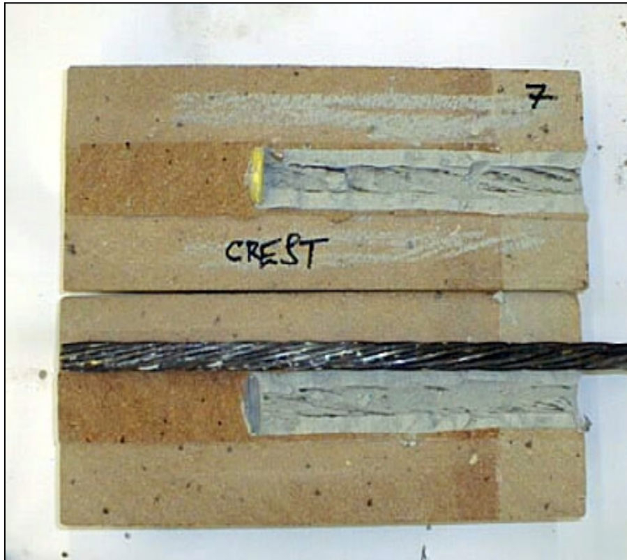
UNBULBED NOTCHED STRAND IN SOUTH AFRICAN CABLE ANCHOR GROUT (TEST 7)
