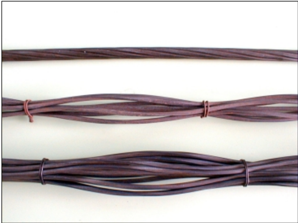
FIGURE 3.1 SINGLE 7 WIRE DYFORM STRAND (top) SINGLE BIRDCAGED CABLEBOLT (centre) DOUBLE BIRDCAGED CABLEBOLT (bottom)
