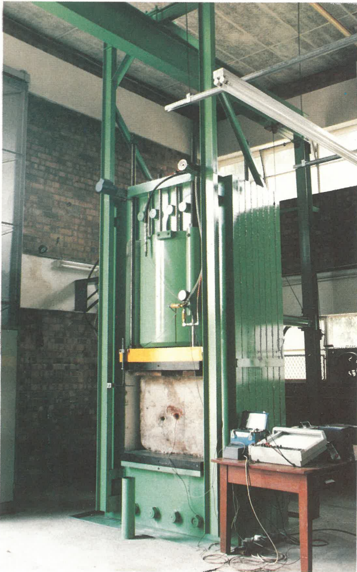
The recently constructed 25 MN compression test rig is shown in the photograph. To obtain a measure of the strength of rock which has numerous joints, fairly large specimens need to be tested. The rig is capable of loading large rock specimens to failure so as to determine their strength.
