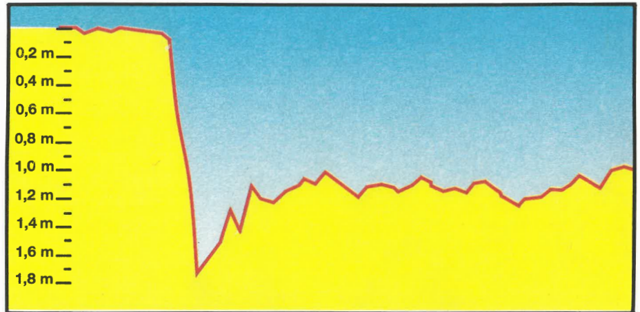
Graph of surface subsidence above a shallow longwall panel showing vertical movements along the centre line of the panel. A noticeable feature is that initial subsidence, which takes place at the initial goaf break, is of the magnitude of 1,75 m. Thereafter it averages at around 1,1 m.
