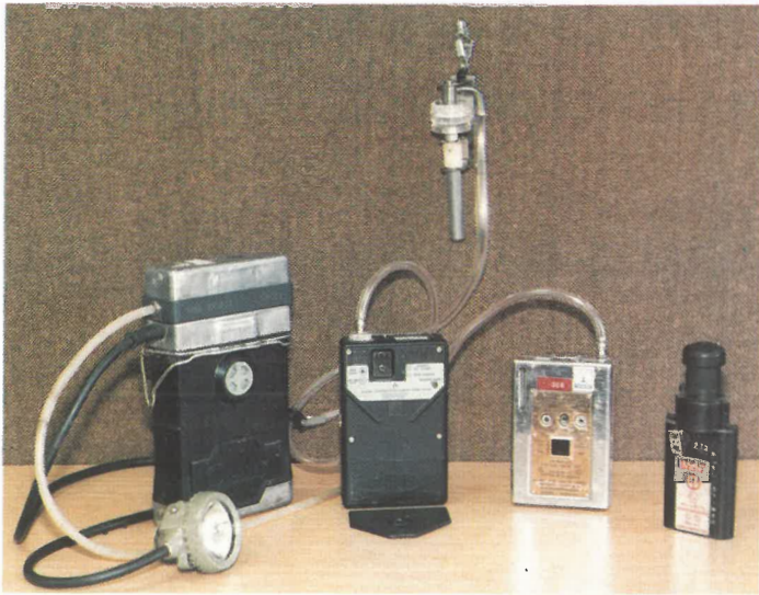
The four personal gravimetric samplers evaluated. During the trial, the performance of the personal gravimetric samplers was monitored over 550 shifts with regard to reliability, robustness, worker acceptance, servicing and repairs. The samplers were also tested in the laboratory following the underground trials, where their performance in a dust chamber was measured against international standards.
