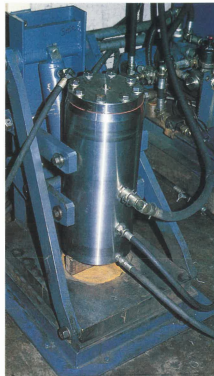
The high speed seal and bearing test unit simulates the sliding velocities and frequencies found in a water powered impact hammer. The unit can be run on clear water and is used to examine the wear characteristics and design features of various bearing and seal materials.
