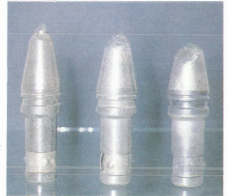
The difference between a blunt and a sharp pick can be clearly seen. During the underground tests investigating pick wear, particular attention is being given to identifying the characteristics of the pick and its location on the cutting drum. Each pick's loss of mass is measured and the wear is graded visually in terms of change in geometry. A geological assessment of the coal seam at each location and a collection of samples for size analysis are also being made.
