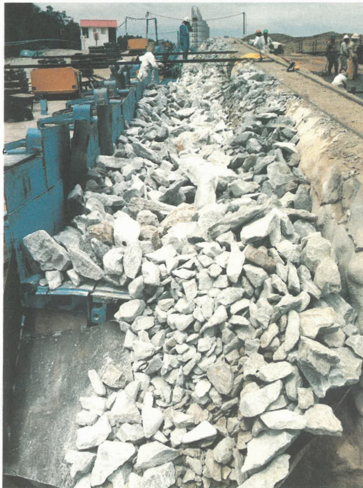
The integrated mechanized mining system for stopes mined with blasting undergoing surface trials at West Rand Consolidated gold mine.
