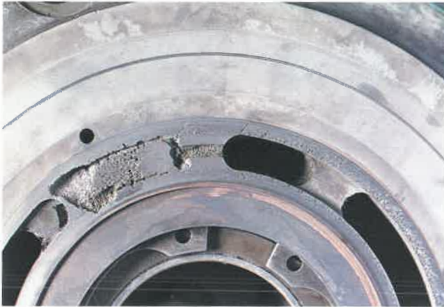
A new port-plate (right) for a hydraulic axial piston pump; after running for 2 500 h on dilute oil and water emulsion it was found to have deteriorated because of cavitation erosion (left).
