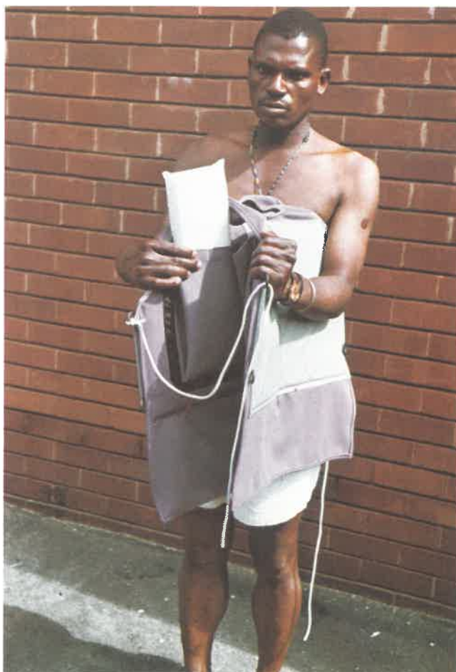
Microclimate suit showing insertion of block of dry ice.
