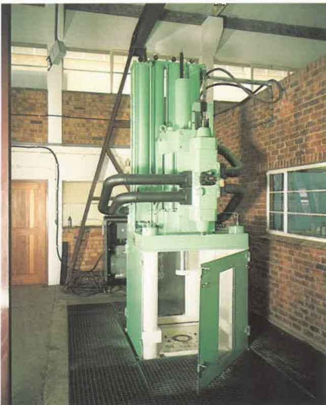
The new 1,8 MN servo-controlled prop-testing machine.
