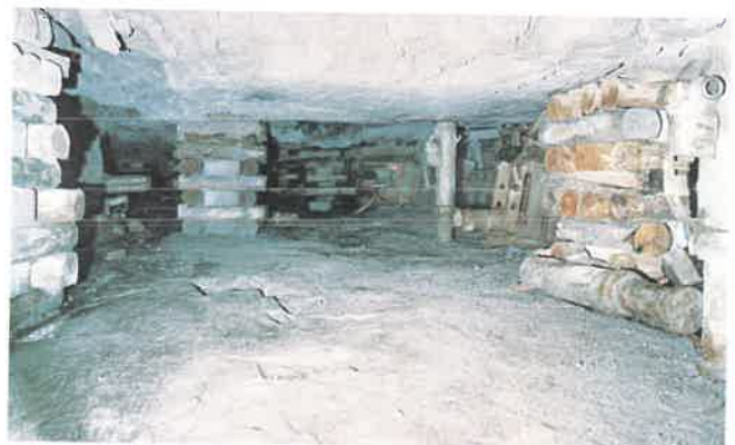
Smooth footwall resulting from the presence of favourable parting planes in a stope mined by blasting. The stope was cleaned using the reciprocating flight conveyor.
