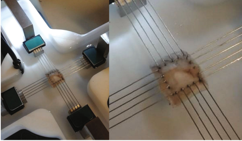
FIGURE 2: Experimental set-up of porcine sclera tissue subjected to biaxial tensile loading (Bio-Tester 5000 from CellScale) (Waterloo, Canada). The hooks (BioRakes) were utilised in securing the sclera tissue and were punched thoroughly before they were inserted into the warm bath of isotonic solution 9.0 g/l at pH of 5.5 at a temperature of 37°C.
