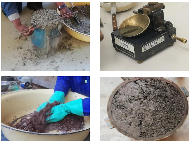
Figure 5: Laboratory pictures: Density (top left), Atterberg testing (top right), Mixing of sample (bottom left), Compaction (bottom right)
