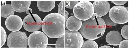
Figure 3. Morphological representation of a) virgin and b) recycled Ti-6Al-4V ELI powder.
