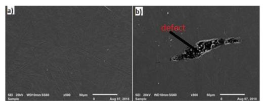
Figure 4. SEM micrographs of the sample built with virgin powder a) and built with recycled powder b).
