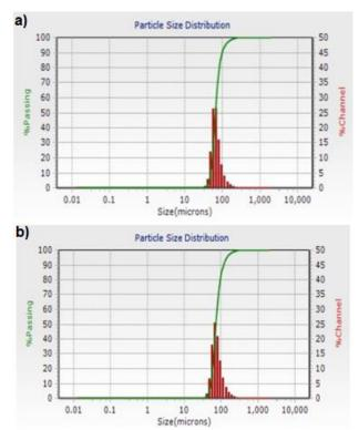
Figure 2. Particle size distribution of a) as-received virgin powder and b) recycled powder.
