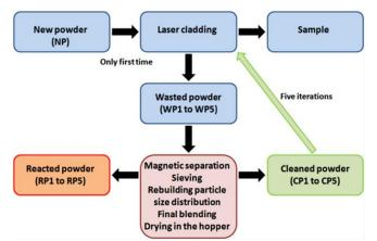
Figure 1. Schematic illustration of the powder recycling procedure.
