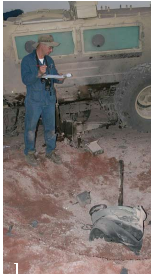
1: Assessments done at a CSIR test facility of the damage caused by a mine to an armoured carrier.
