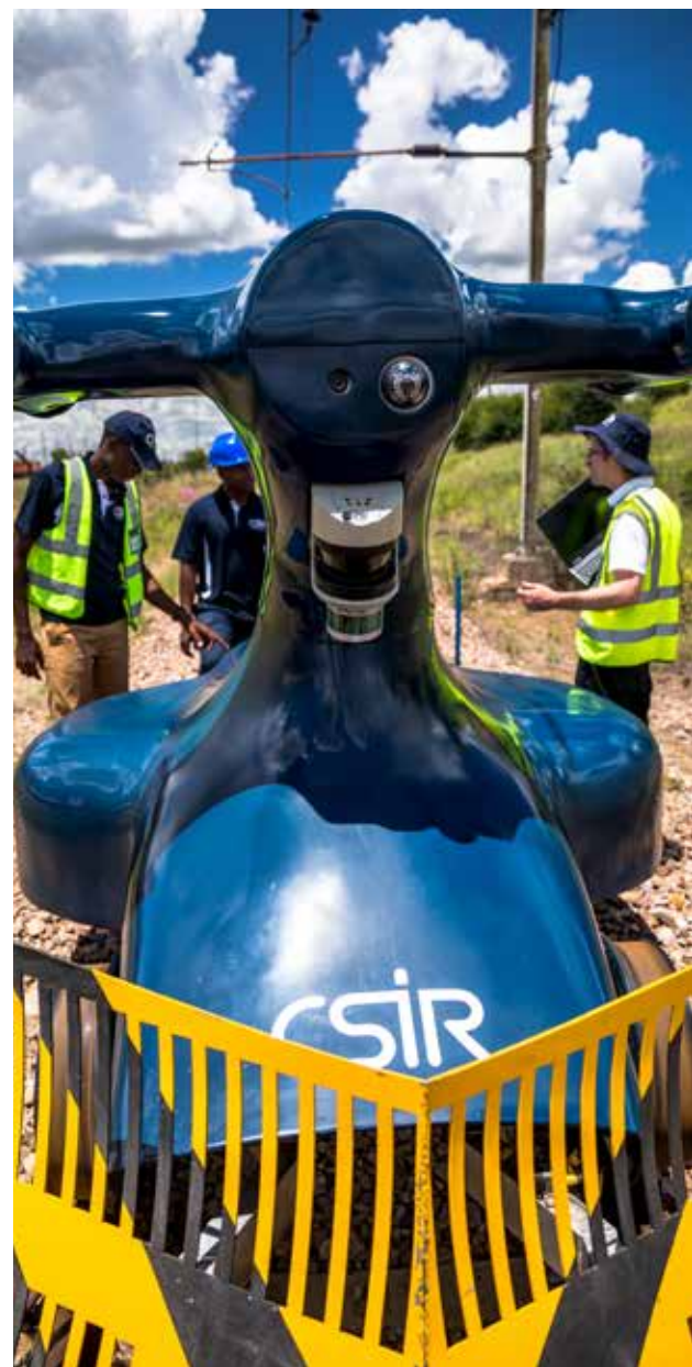
Field trials of a rail inspection device that travels ahead of locomotives and warns train drivers of dangers ahead.
