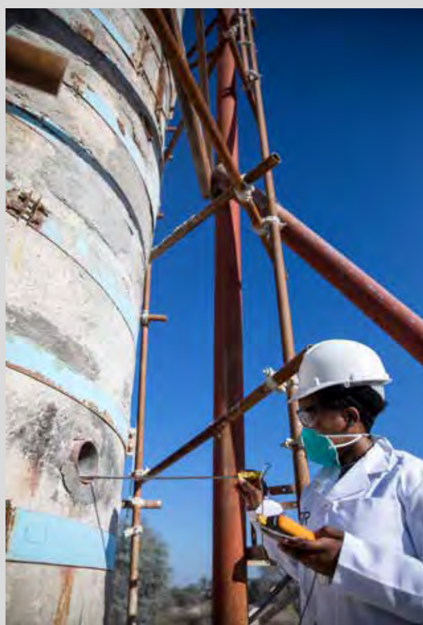
CSIR researcher Zonke Dumani tests kaolinitic clays used to produce metakaolin in a vertical shaft kiln at the Roedtan Leo Mine in Limpopo. The CSIR is in the process of setting up an industrial-scale pilot plant to produce metakaolin.
