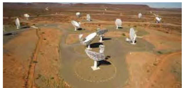
An aerial view of the MeerKAT core at the SKA project's Losberg site in the Karoo, in the Northern Cape. The MeerKAT radio telescope array will consist of 64 antennas which will be integrated into the first phase of the SKA project. Image courtesy SKA South Africa
