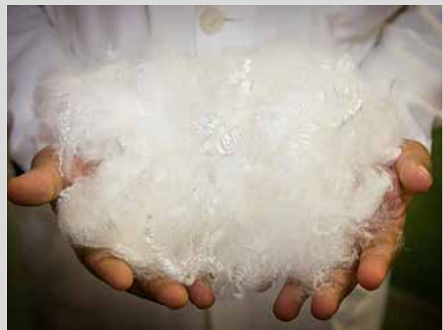
Polyacrylonitrile used to manufacture fabric for filter bags.
