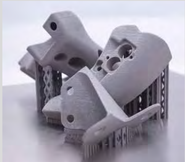
The Aeroswift team produced two different flight grips (the condition lever grip and throttle grip) for the South African developed AHRLAC aircraft. The titanium metal part on the far right of the top image is a fuel pylon bracket developed for a commercial aircraft. The bottom image shows the parts from a different angle.
