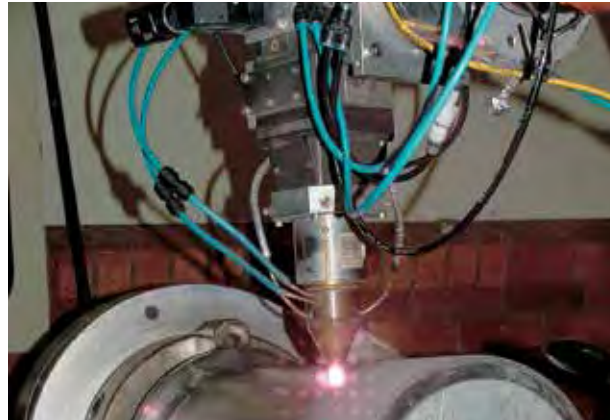
Laser cladding of a roll using laser technology.
