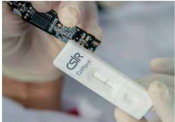
The low-cost E. coli detection device, ColiSpot.
