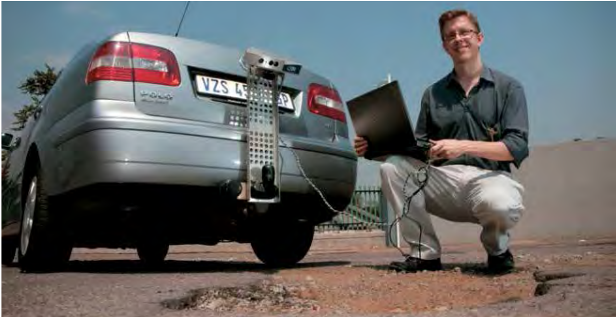
CSIR engineer Deon Joubert calibrating a prototype of the visual surveying platform.
