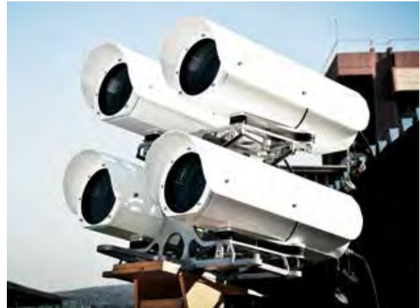
The multi-spectral camera system has four separate sensor units, each with an optical zoom lens and non-overlapping spectral filters and polarising disks.
