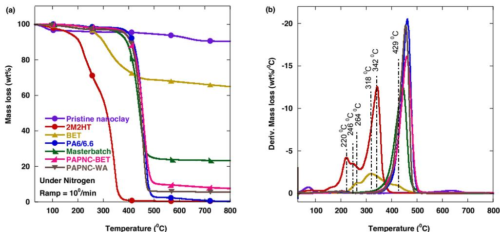
**FIGURE 1.** (a) TG and (b) DTG of the neat materials and polymer nanocomposites.
