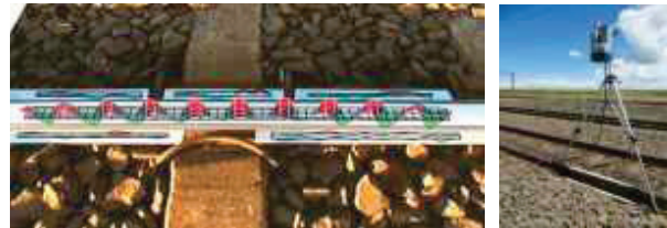
Figure 4. Scanning laser vibrometer measurement of ultrasonic guided waves.
