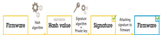
Fig 2: The process of signing firmware[14].
