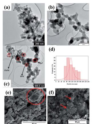
Fig. 2 TEM images of (a)  $Fe^0$ -PANI, (b)  $Fe^0$ -PPY, (c)  $Fe^0$ -PPY/PANI (d) particle size distribution of  $Fe^0$  nanoparticles in  $Fe^0$ -PPY/PANI and SEM image of (e) PPY/PANI and (f)  $Fe^0$ -PPY/PANI.
