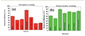
Fig. 5 Removal efficiencies of BPA using the various materials by (a) adsorption and (b) Fenton reaction. Experimental conditions: 50 ml of 50 ppm BPA, 25 mg of catalyst or adsorbent and 15 ppm  $\rm H_2O_2$  for only Fenton reactions.
