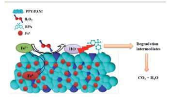
Fig. 13 Advanced Fenton reaction mechanism for the degradation of BPA using  ${\rm Fe^0}$ -PPY/PANI.
