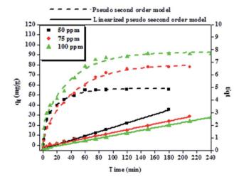
Fig. 8 Adsorption kinetics and the pseudo-second-order kinetic plot of BPA adsorption onto 50 mg of PPY/PANI. Experimental conditions: 200 ml of various concentrations of BPA (50, 75 and 100 ppm) at pH 6.0 and at 23 °C.
