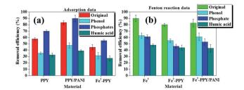
Fig. 6 Removal efficiencies of bisphenol-A in the presence of other contaminants using the various materials by (a) adsorption and (b) Fenton reaction. Experimental conditions: 50 ml of 50 ppm BPA, 25 mg of catalyst or adsorbent and 15 ppm  $\rm H_2O_2$  for only Fenton reactions.
