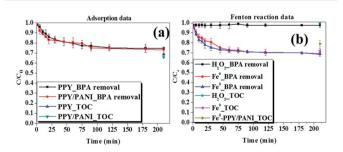
Fig. 7 Removal efficiencies of bisphenol-A and TOC using various materials by (a) adsorption and (b) Fenton reaction. Experimental conditions: 200 ml of 50 ppm BPA, pH 6 for adsorption experiments and pH 3 for Fenton reactions, 100 mg of adsorbent or Fenton catalyst and 25% of sewage-water.
