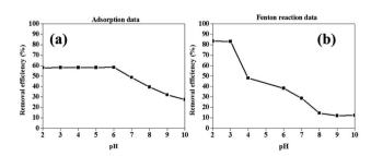
Fig. 4 Effect of pH on the (a) adsorption of BPA using PPY and (b) Fenton degradation of BPA using  $Fe^0$ . Experimental conditions: 50 ml of 50 ppm BPA, 25 mg of catalyst or adsorbent and 15 ppm  $H_2O_2$  for only Fenton reactions.
