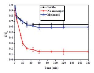
Fig. 11 Effect of methanol and potassium iodide on the removal of BPA. Experimental conditions: 200 ml of 50 ppm BPA at pH 6 with 100 mg  $\rm Fe^0$ -PPY/PANI and 5 mM KI or 350 mM methanol.
