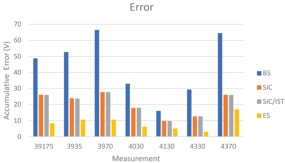
Figure 9: Average errors obtained from various temperature compensation strategies when applied to ultrasonic measurements from an operational railway line.
