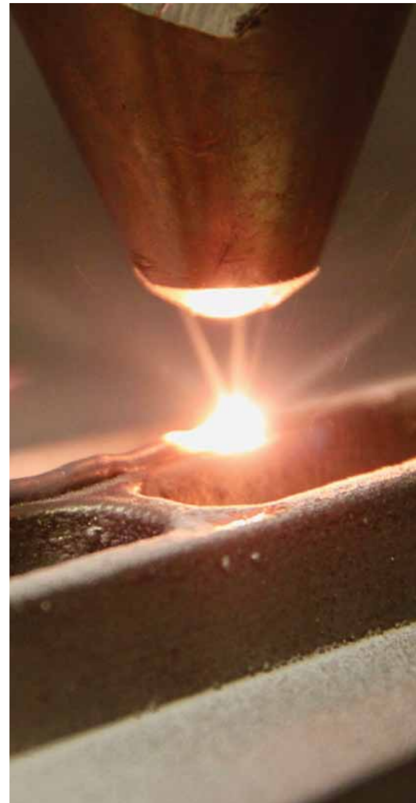
The CSIR’s laser cladding capability is a laser refurbishment process for worn, damaged or faulty components. The process is used to repair turbine blades, press tools and shafts.
