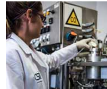
▲ Above: (from left) Preparation of a polymer-probiotic premix; adding the premix to a high-pressure CO 2 vessel and the encapsulated probiotic.
