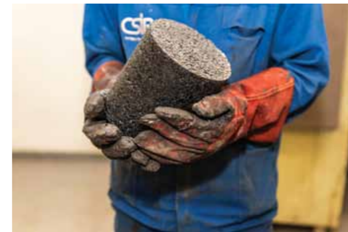
◀ Left: A sample of crushed glass. The use of crushed glass is being studied as a substitute to natural aggregate in asphalt mixes. ▲ Above: Laboratory-compacted glass-asphalt test samples.
