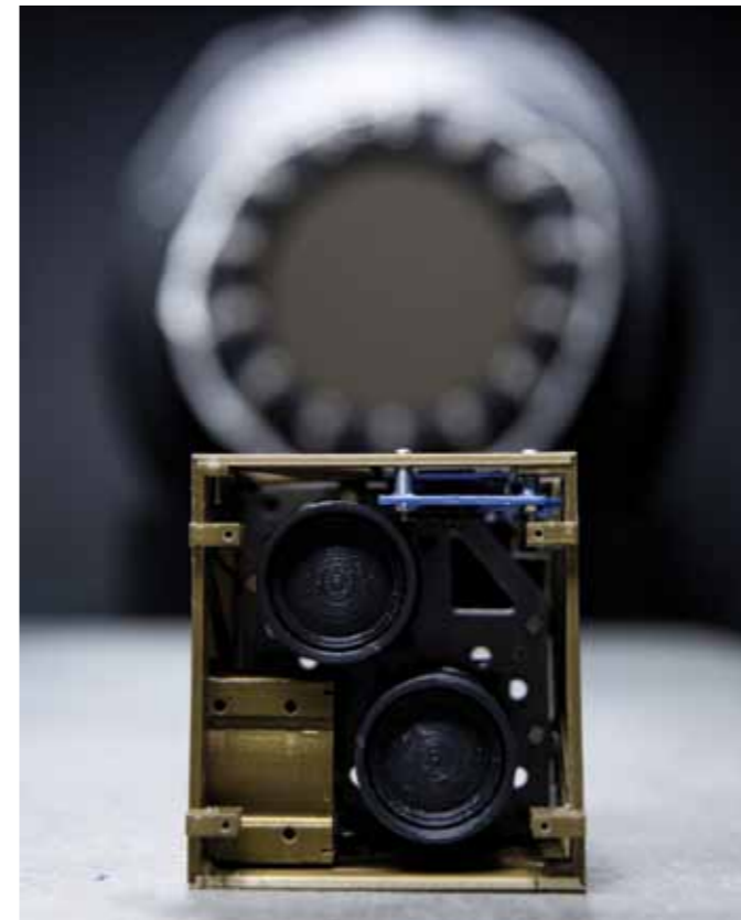
▲ Above: (left) A 3D printed plastic model of the K-line camera. (Right) A mock-up of the 30 x 10 x 10 cm ZA-CUBE-2 satellite with the K-line camera at the bottom of the cube stack.
