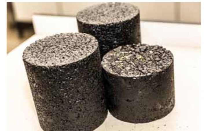
◀ Left: A sample of crushed glass. The use of crushed glass is being studied as a substitute to natural aggregate in asphalt mixes. ▲ Above: Laboratory-compacted glass-asphalt test samples.
