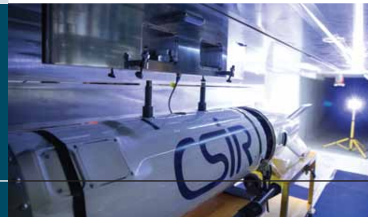
▼ Below: (left) The ram air turbine underwent tests in the CSIR's medium speed windtunnel to validate the levels of power it was able to generate over the full flight envelope of the pod. (Right): The pod was also tested on a Mirage F1 fighter plane.
