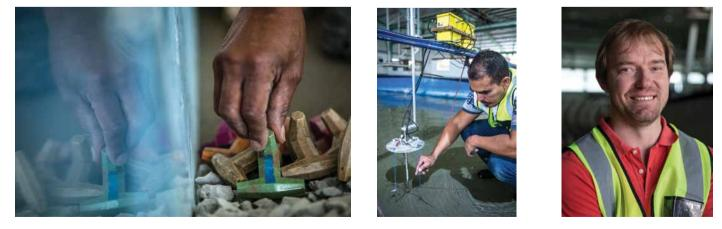
Left: The CSIR's coastal and hydraulics laboratory is one of four facilities of its size in the world, where scale models are built to test harbour and coastal engineering design. A Above (centre): Rafick Jappie sets up a wave-height gauge to measure wave height and wave direction.
