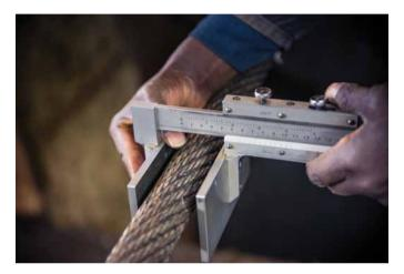
platform. Wire ropes – up to 160 mm in diameter and with a 1 500 ton breaking-strength – have been tested for heavy lifting and marine industry application.
