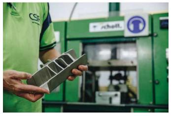
▲ Left: A three-chamber vacuum casting furnace. (Inset) A commercial micro turbine stator and rotor casting produced at the CSIR. ▲ Above: The CSIR's Pierre Rossouw with a newly installed de-waxing boiler for wax removal from moulds. (right) A titanium-casted aileron produced in the facility. An aileron is a hinged flight control surface used on fixed-wing aircraft.
