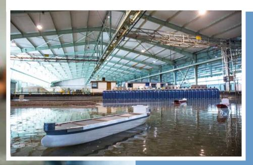
The CSIR's coastal and hydraulics laboratory is used as a design tool where engineers and scientist can build smallscale versions of planned coastal infrastructure and its surrounding area. The coastal processes and wave conditions are then simulated to test the performance of the planned infrastructure as well as the unintended impact such structures may have on the surrounding coastline and coastal processes. The impact of future climate change can also be tested in these physical models.
