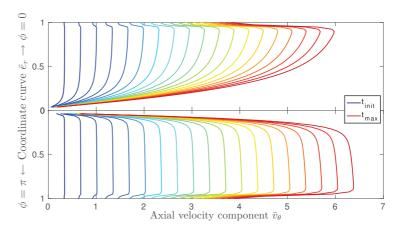
Ventriculoperitoneal shunt implanted into human body for cerebrospinal fluid drainage [II] (left) & Expansion throughout time of the axial velocity component evaluated at the end of the ventricular catheter and induced by an upstream pressure force (right).
