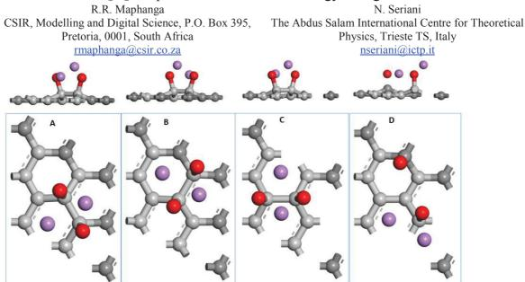
Figure 1: Final configurations of Li<sub>2</sub>O<sub>2</sub> adsorbed at A, B, C and D positions of graphene layer. Side and top views of optimized structures of the Li<sub>2</sub>O<sub>2</sub> adsorption configurations on graphene are shown with grey, red and purple balls representing carbon, oxygen, and lithium atoms respectively.
