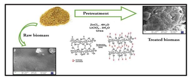
Figure 1: Scanning electron micrographs of raw biomass and ZnCl<sub>2</sub>.4H<sub>2</sub>O treated biomass
