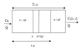
Figure 1: Ammonia-nitrogen concentration through a plug flow cell.
