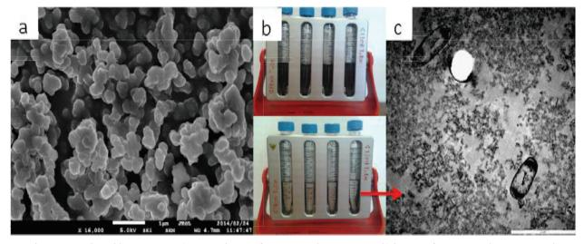
Figure SEQ Figure  $\$  ARABIC 4: a) A SEM image of PPy-COOH/ Fe<sub>3</sub>O<sub>4</sub> MNCs, b) images of PPy-COOH/ Fe<sub>3</sub>O<sub>4</sub> MNCs in suspension before and after magnetic separation and c) a TEM micrograph of antibody-labelled PPy-COOH/ Fe<sub>3</sub>O<sub>4</sub> MNCs bound to E. coli cells. Insert: Magnified E. coli cell
