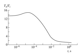
**Fig. 4.** Ratio of the heating temperatures of the outer (o) and inner (i) surfaces of the absorbing layer in relation to the irradiation time at the irradiance on the laser beam axis  $5 \times 10^5 \text{ W/m}^2$ .
