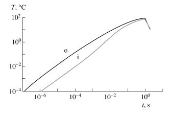
**Fig. 3.** Heating kinetics of the outer (o) and inner (i) surfaces of the absorbing layer at the irradiance on the laser beam axis  $5 \times 10^5 \text{ W/m}^2$ .
