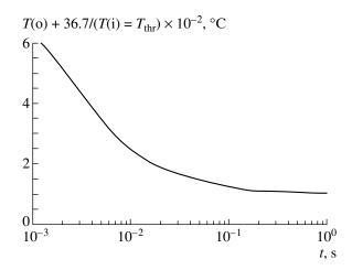
**Fig. 6.** Maximal temperature of the outer surface of the absorbing layer corresponding to the threshold coagulation conditions of the inner surface plotted as a function of the exposure time.
