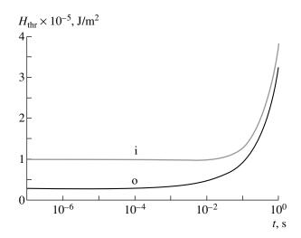
**Fig. 5.** Threshold radiant exposure  $(H, J/m^2)$  of the inner (i) and outer (o) surfaces of the absorbing blood layer in relation to the laser pulse duration.
