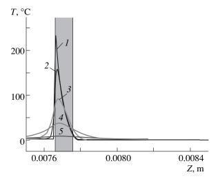
**Fig. 2.** Fragment of the axial temperature distribution in a model structure irradiated by rectangular laser pulses with the duration  $\tau = (I) \ 10^{-5}$ ,  $(2) \ 10^{-3}$ ,  $(3) \ 10^{-2}$ ,  $(4) \ 0.1$ , and  $(5) \ 1$  s. The position of the blood layer is shaded. The radiant exposure H in all cases is  $5 \times 10^4 \ J/m^2$ .
