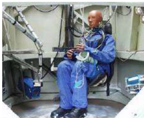
Figure 2.13: The inside of the TROSS™ with a Hybrid III ATD and instrumentation (Reproduced from Bir et al., 2006)
