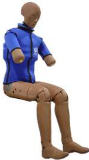
Figure 2.4: EuroSID with rib extension male ATD (Reproduced from Humanetics Innovative Solutions, 2010)
