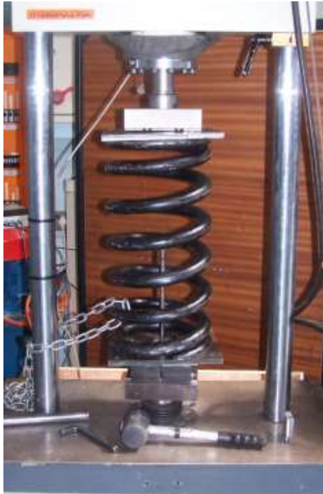
Figure 3.4: Compression tests of new spring for MLLI
