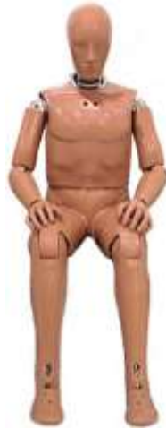
Figure 2.3: Hybrid III 50th percentile male ATD (Reproduced from Humanetics Innovative Solutions, 2010)
