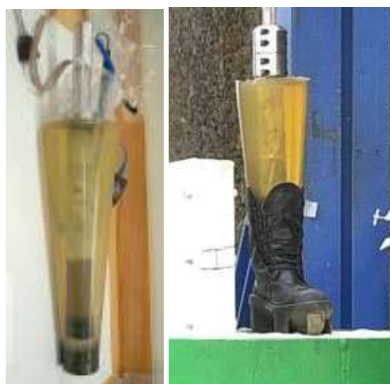
Figure 2.28: Simplified lower leg (Reproduced from Cronin et al., 2003)
