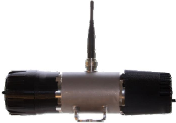
Fig. 1. The GS01 Wireless Infrared Hydrocarbon Gas Detector. Battery compartment to the left, sealed electronics housing in the middle and measurement volume to the right, protected with a weather protection. Antenna on the top, and mounting foot in the bottom.
