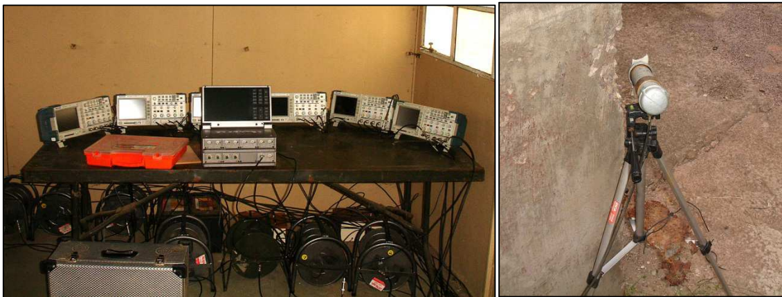
Figure 6: Oscilloscopes and Graphtec used for Data Capture (left) and Light Sensitive Trigger System (right).
