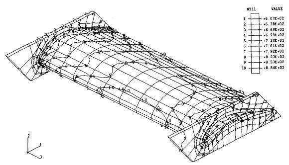
Fig. 1. Blade metal temperature distribution.
