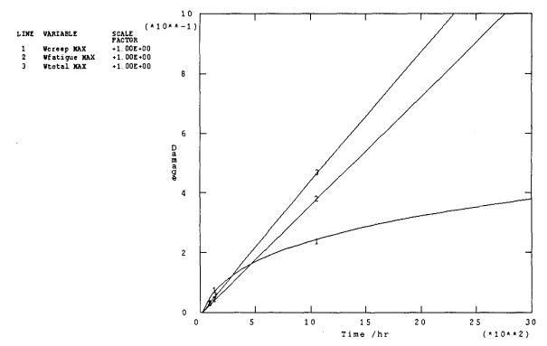
Fig. 3. History plot of the maximum damage parameters.
