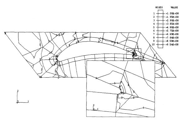
Fig. 2. Von Mises stress distribution.
