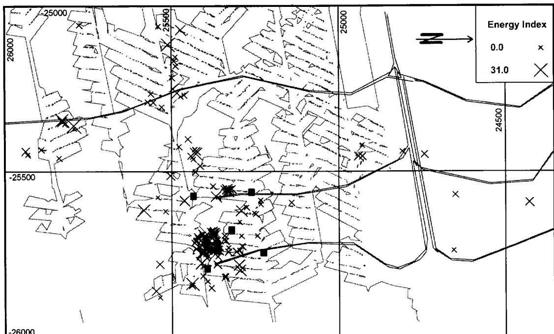
Figure 12. Energy index distribution in the vicinity of the PSS installation.
