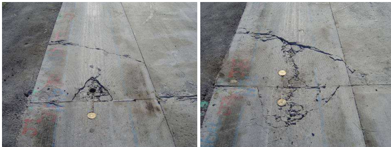
Figure 11. End of life at the two joints of section 1, loaded to failure
