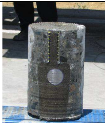
Figure 2: Slab positioning and core showing dovetail slot/dowel bar connection
