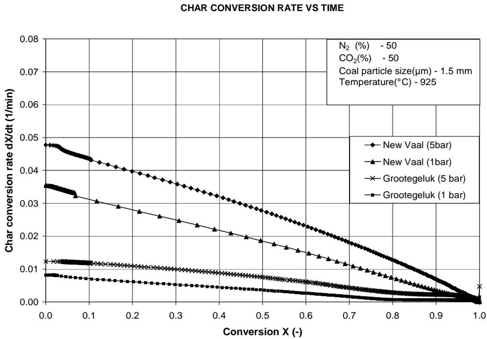
Figure 9: Char conversion rate vs conversion at 1 and 5 bar pressure.
