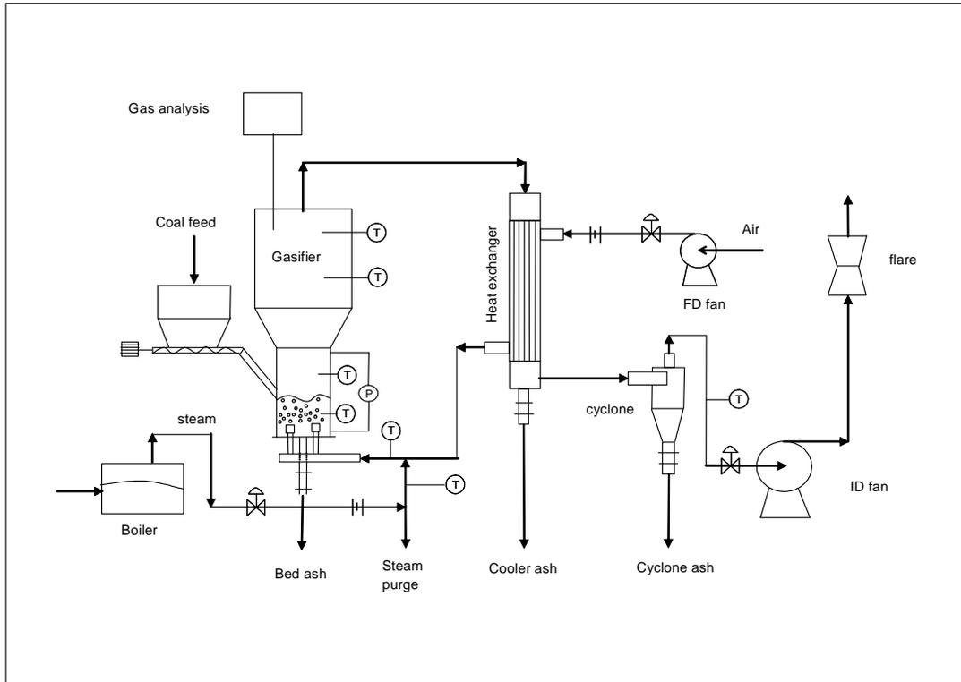
**Figure 10:** Flow diagram of the CSIR Pilot fluidised bed gasifier.
