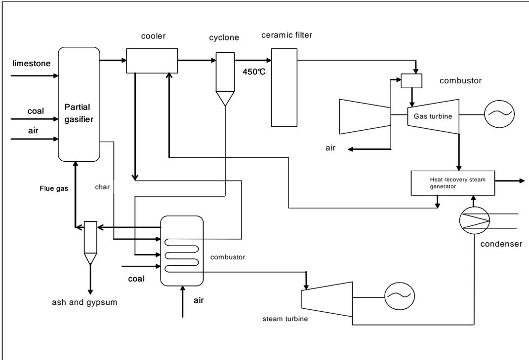
**Figure 3:** Hybrid gasification combustion system.
