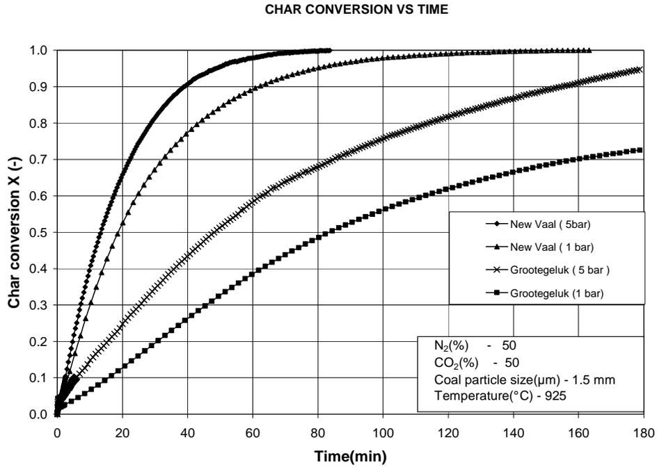
Figure 8: Char conversion vs time at 1 and 5 bar pressure.
