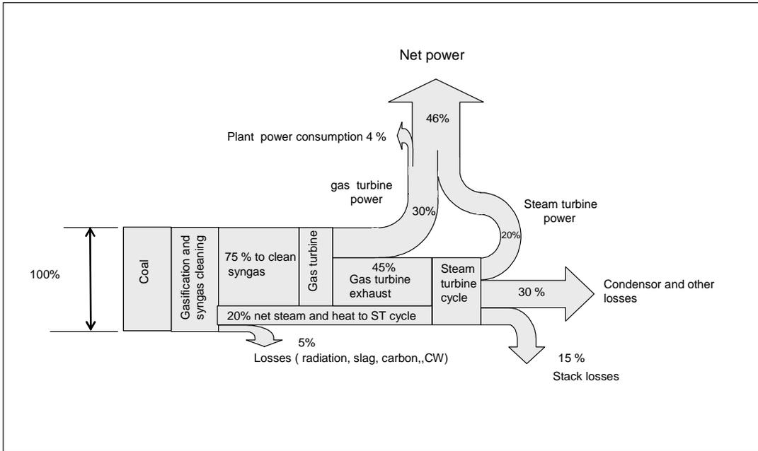
**Figure 2:** Energy flows in aIGCC power station.
